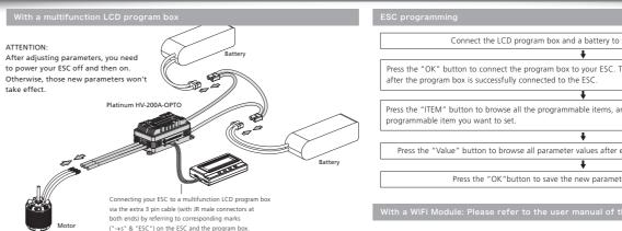
Connect the LCD program box and a battery to your ESC as shown above
